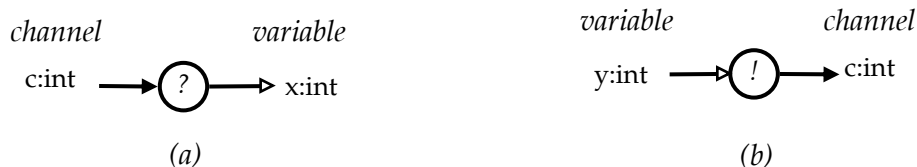
Figure 3-36 Primitive communication processes on data channels: (a) data channel input, i.e. channel to variable, (b) data channel output, i.e. variable to channel.
